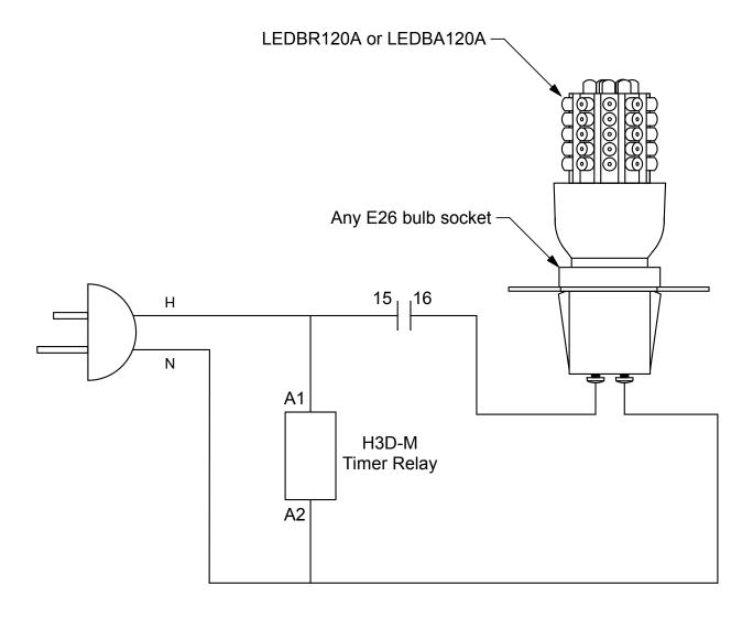
Hook up for flash operation using timer. Example shown employs Ingram Products H3D-M multifunction timer relay. (Sold separately.) Set Mode for B or B2. (Flasher settings.) Flash rate can be adjusted from 1/10th of a second to 100 hours.
