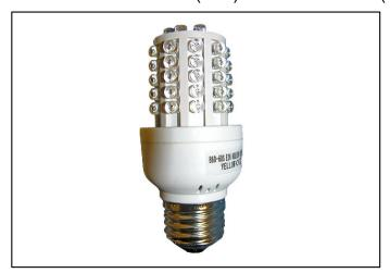
Ingram has designed a variety of daylight visible, low power LED bulbs for your alarm needs. The LEDBR120A and LEDBA120A fit Ingram's LX25 alarm light. In fact, these screw-in type bulbs fit any standard medium base (E26) socket. Unlike incandescent bulbs that fail catastophically when the filament burns out or is broken, LED matrix designs will continue to light, should a single LED or a row fail.
