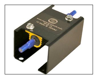
The mini space heater is designed for interior enclosures where space is at a minimum, and a limited amount of heat is required. Use it to keep the temperature inside an enclosure several degrees above the external ambient temperature and above the dew point. Keep your electrical equipment on line by preventing corrosion due to condensation. Contact our engineering department for specifications for the proper AHC or MHS model used in other types of enclosures (Aluminum, Fiberglass, etc.).
